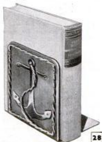
Photo above and detail and photo below show nautical book ends of riveted construction. Length of twisted wire provides "rope"
